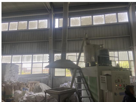
涉及粉尘工序得集气罩
