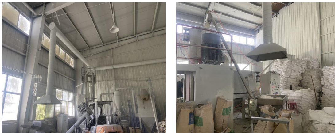
涉及粉尘工序得集气罩
